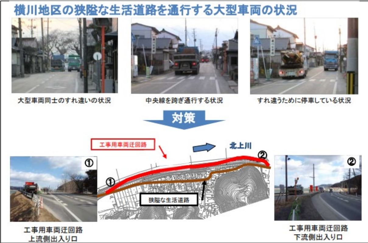
Figure 5-6-27 Setting up a detour for construction vehicles in the Yokokawa District
