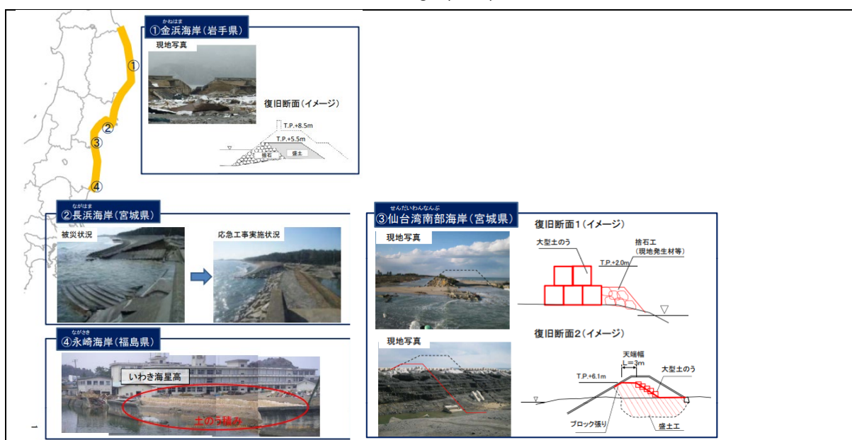
Figure 5-6-5 Basic approach to disaster recovery of coastal levees experiencing destructive levels of damage (draft)
