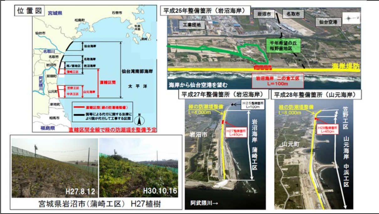
Figure 5-6-9 Construction of a "green seawall" on the Southern Sendai Coast to serve as a model
