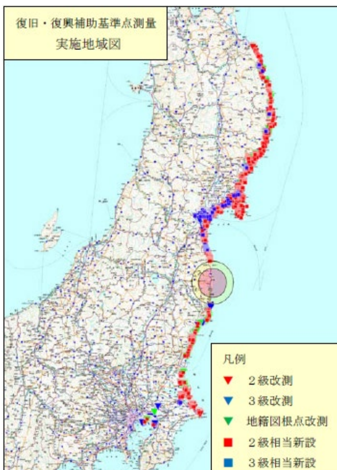
Figure 3-2-10 Areas for Reconstruction and Reconstruction Auxiliary Control Point Surveys
