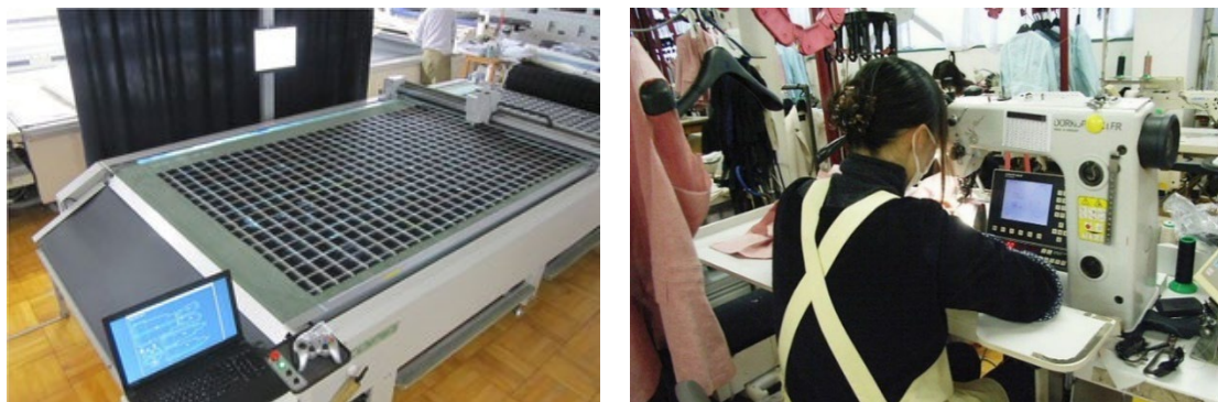
Photos: State-of-the-art pattern cutting CAM equipped with a TV camera (left) Specialized sewing machine with built-in computerized sleeves (right) (Source: Iwate Moriya website)
